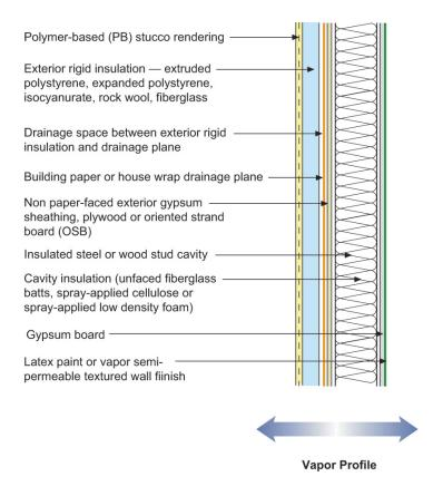
Figure 13: Frame Wall With Exterior Rigid Insulation With Cavity Insulation and Stucco
