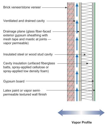
Figure 7: Frame Wall With Cavity Insulation and Brick or Stone Veneer
