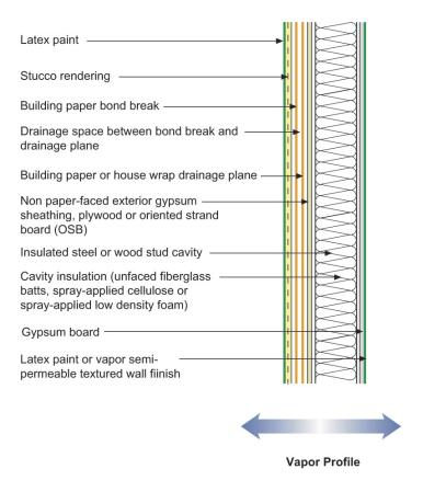
Figure 11: Frame Wall With Cavity Insulation and Stucco
