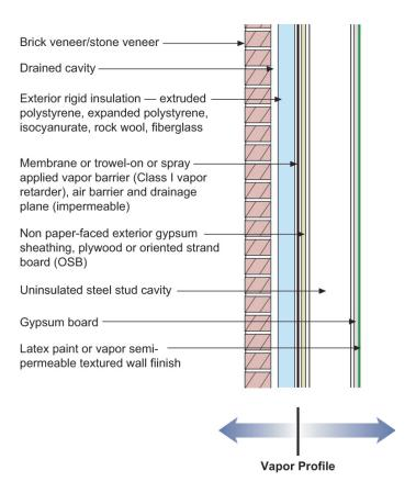
Figure 5: Frame Wall With Exterior Insulation and Brick or Stone Veneer
