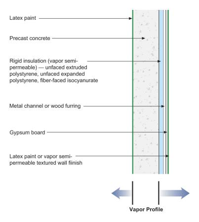
Figure 15: Precast Concrete With Interior Rigid Insulation
